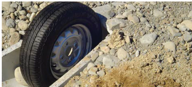
Demonstration of snagging risk of chamfered culvert end
