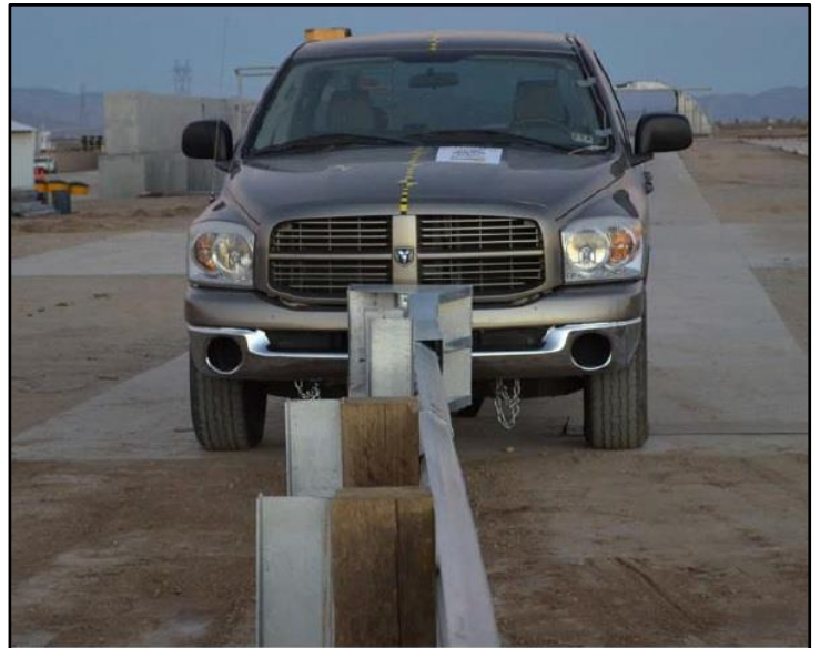
MASH Test 3-33 Set-Up (2270P at 100km/h and 5°)
