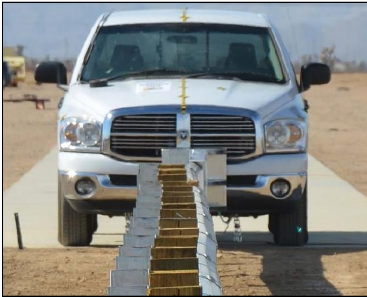
MASH Test 3-31 Set-Up (2270P at 100km/h and 0°)
