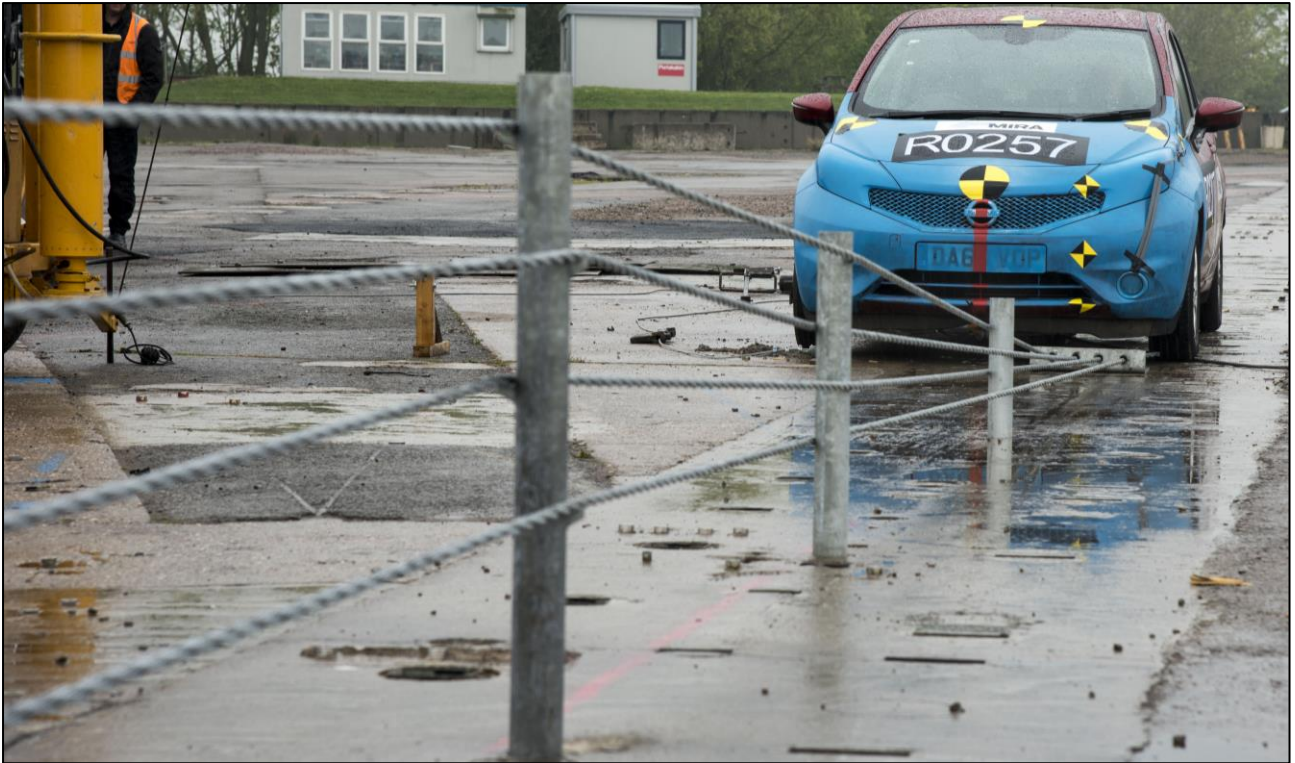
Figure 13: Cable Weave at Terminal
