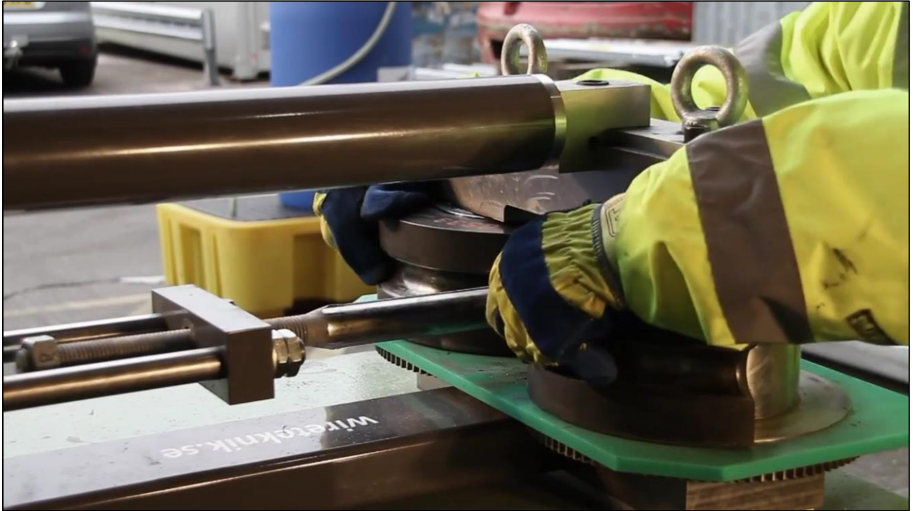
Figure 11: Rotate dies back to starting position after swaging
