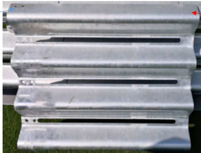
Fig. 22: Side panel description. The holes are located on the front side.
