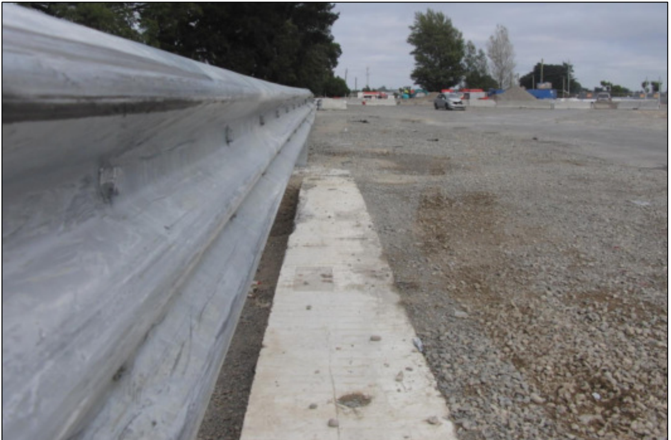
Figure 8: Nil Damage to CrocGuard® Following MASH 4-10 Impact
