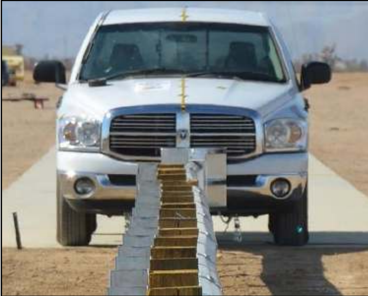
MASH Test 3-31 Set-Up (2270P at 100km/h and 0°)
