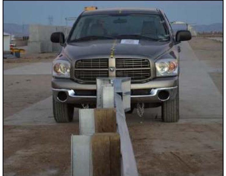
MASH Test 3-33 Set-Up (2270P at 100km/h and 5°)
