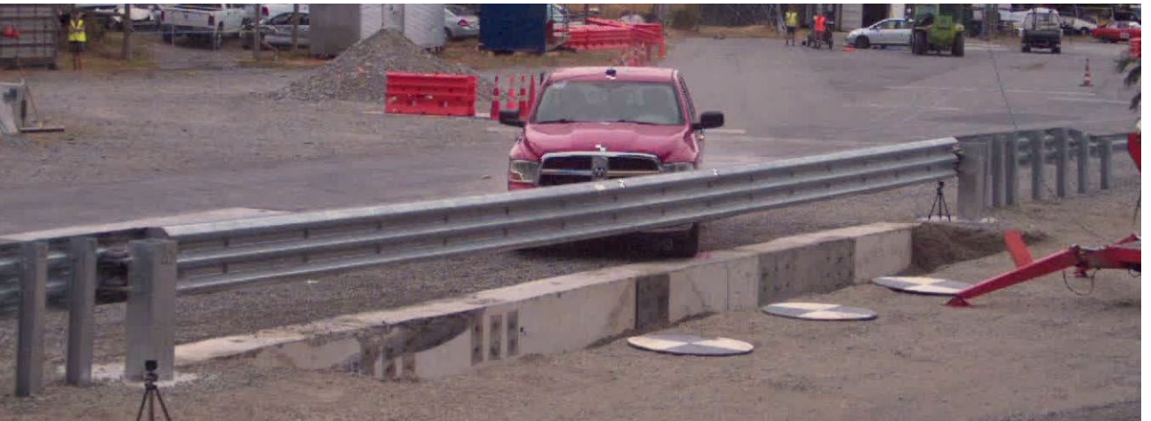
Figure 2: Crash Test Impact: 2270kg Pick-up Truck, 100km/h and 25 degrees
