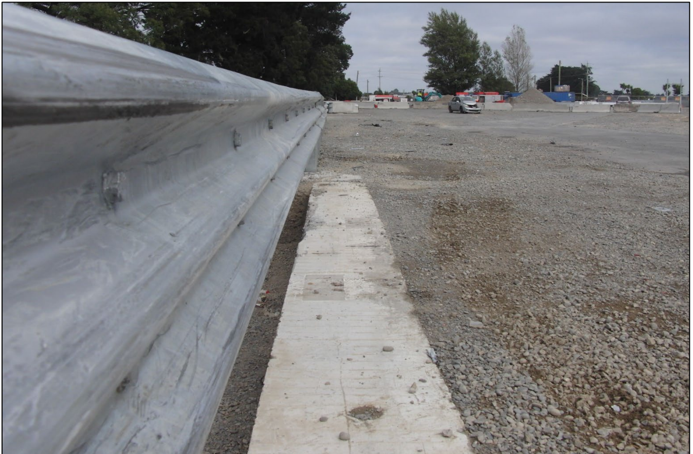
Figure 8: Nil Damage to CrocGuard® Following MASH 4-10 Impact
