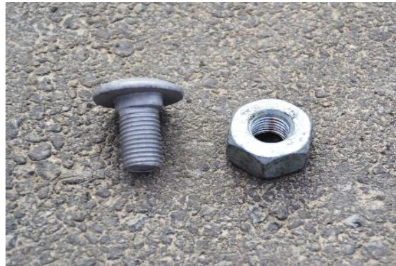
Splice Bolt and Nut
