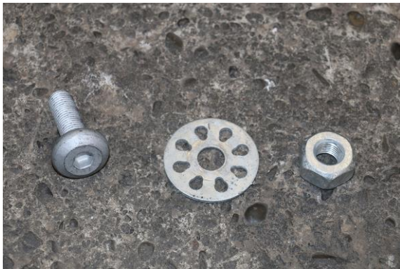
ACP Sentry Barrier Bolt, Washer and Nut
