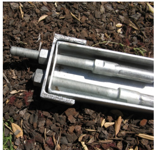
Figure 23. Thread the nuts as shown
