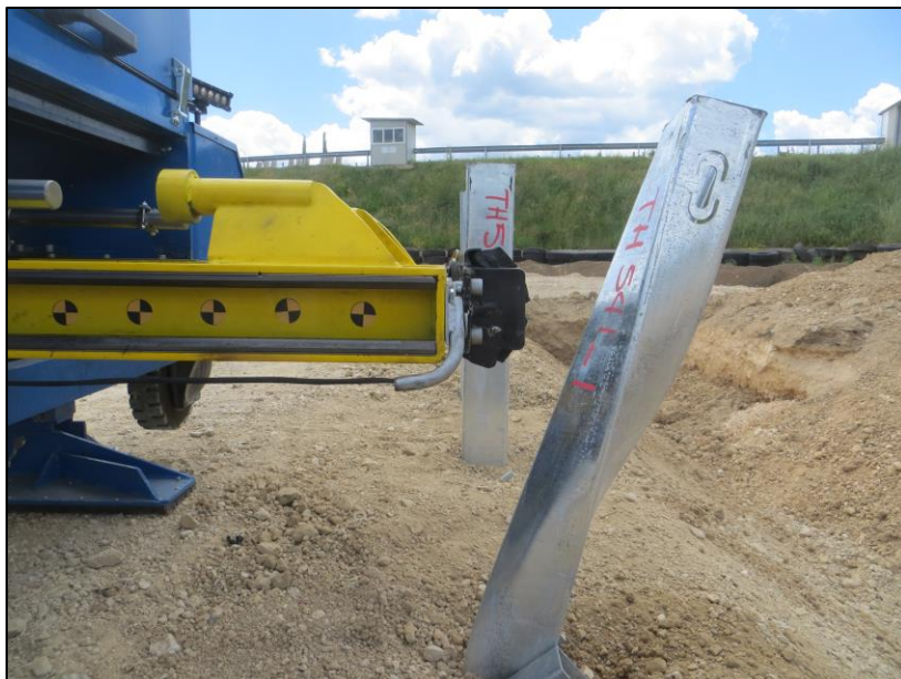
Figure 11: Dynamic Impacts with Mobile THOR Apparatus
