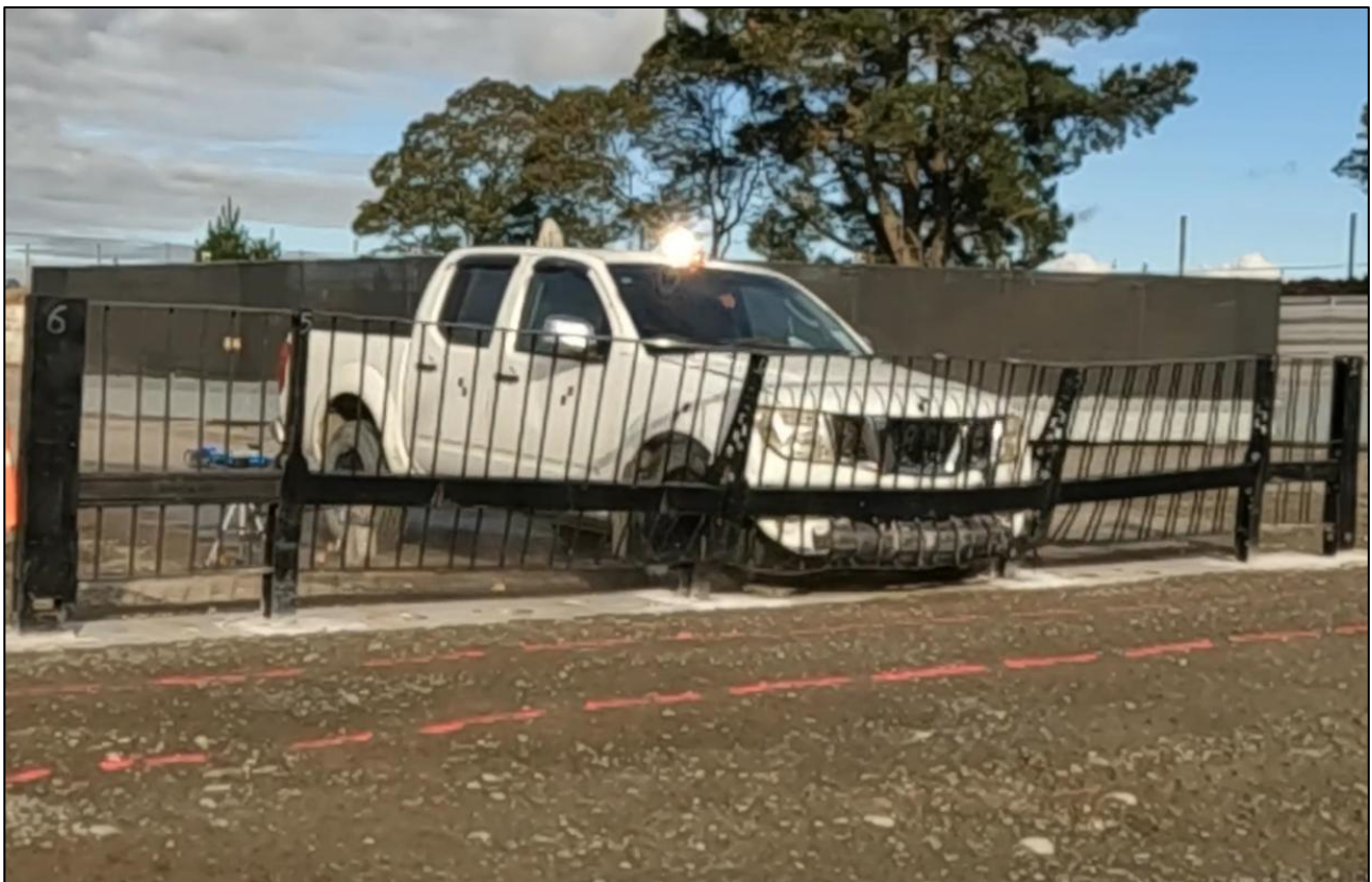
Figure 1: Impact behaviour of ZebraFence®, 2000 kg dual cab utility travelling at 40 km/h and 90-degrees.
